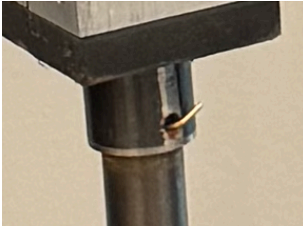
Fig. 33. Shear Pin assembly close-up. Note the large clearance of the shear-pin hole. We suspect this allowed significant deformation of the pin, resulting in different loading conditions than we initially predicted.
