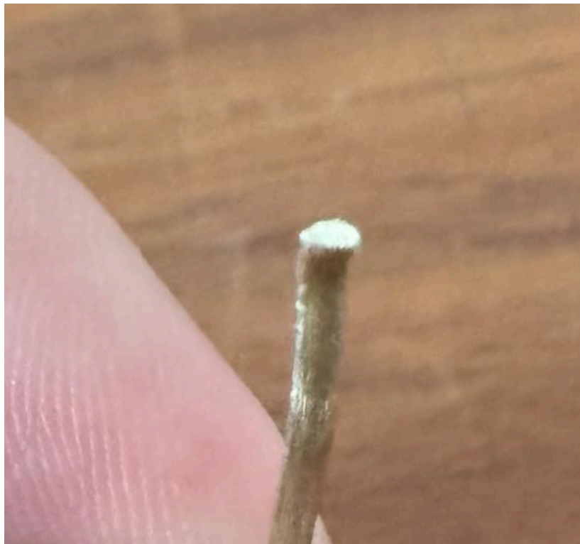
Fig. 32. Picture of cross section of 1/32" shear-pin. Note the non-circular cross-section.
