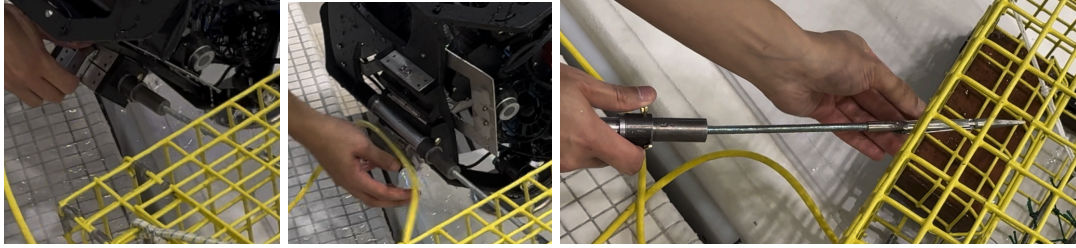
Fig. 38. Left: spear in latch-box immediately after retrieval. Middle: spear being removed from latch box. Right: spear being removed from pot. Entire process completed in <12 seconds.
