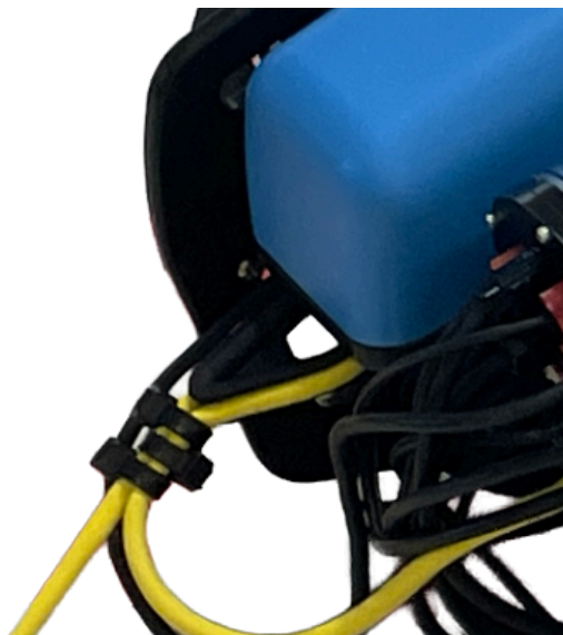
Fig. 16. Picture of the nylon thimble Blue Robotics sells for use as a strain relief.
