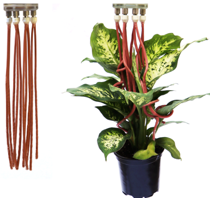
Fig. 21. Depiction of filament-like soft robotic actuator developed by Prof. Kaitlyn Becker [11].
